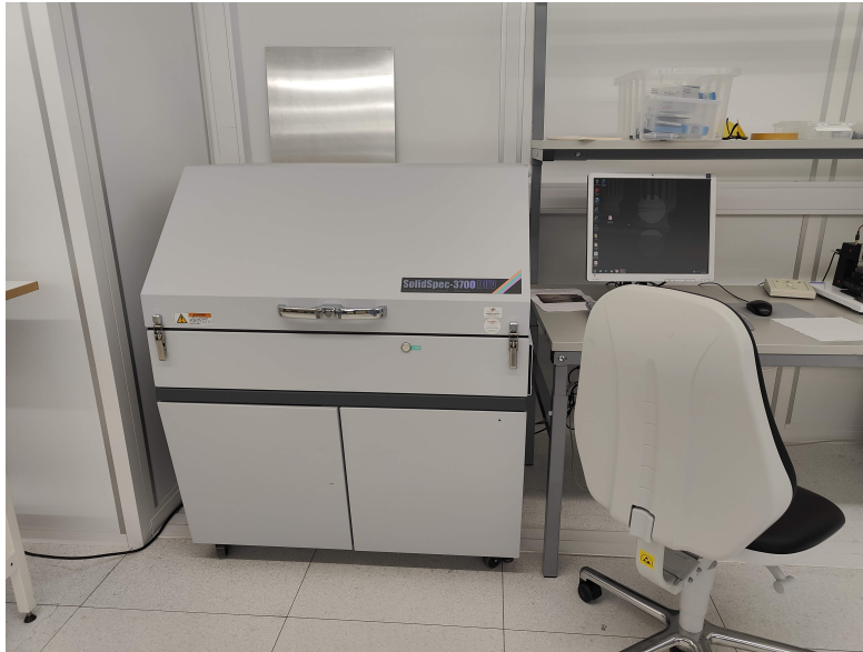
Figure 3.5: Shimadzu SolidSpec-3700 DUV with an integrating sphere found at MiNaLab. Suitable for transmission, reflection, and scattering measurements of thin films.
